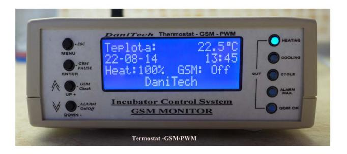
Device is designated for measurement and regulation of temp. and humidity GSM - alarm on the cell phone
